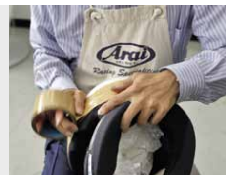
5 All the inner parts of the helmet are now bound carefully together before being inserted
