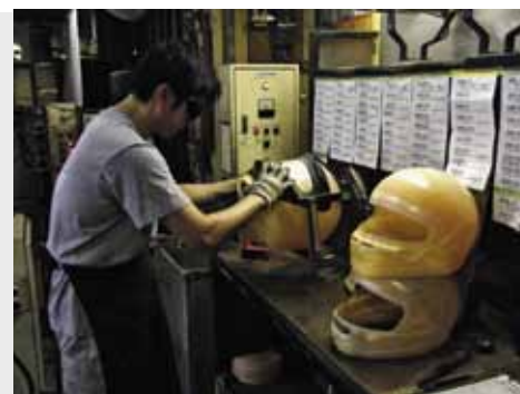
2 With the visor hole and air vent lasered in, the shell is primed and sanded, then sent to be painted
